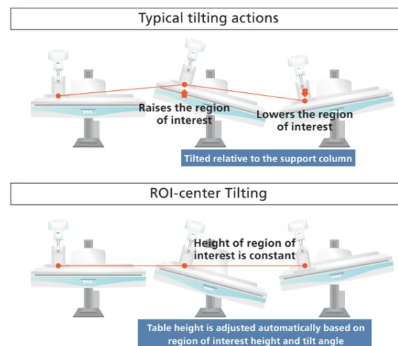
The table can be tilted relative to any reference position. Examinations can be performed without changing the region of interest height, even if the table is tilted.
